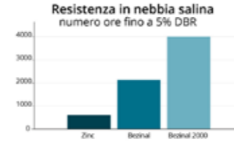
Galvanized Wire Class A - EN10244-2 (according to DIN SS 50021; DIN 50018) DBR Deep Brown Rust - Dark Corrosion
